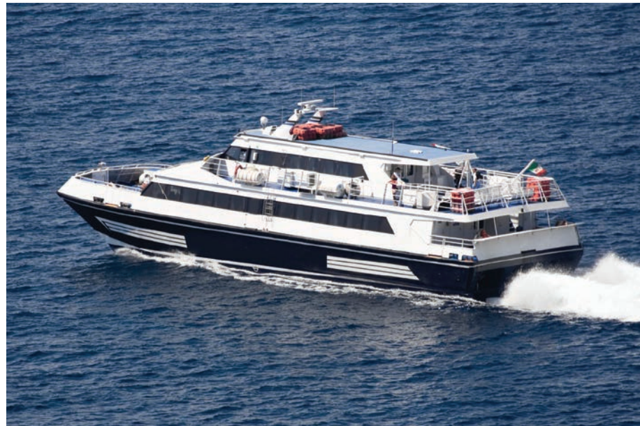
Figure 4.4 Typical fast ferry application of waterjet propulsion
