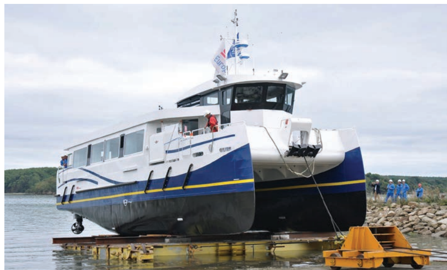
Figure 3.9 Ar Vag Tredan super-capacitor driven ferry [Courtesy stx-Lorient]
