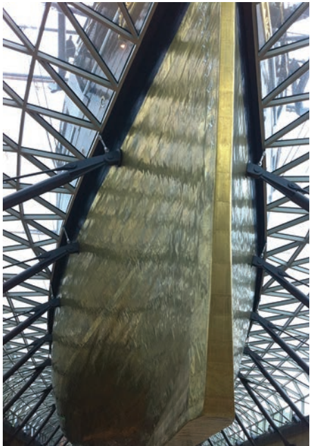
Figure 1.3 Copper sheathing on the hull of the Cutty Sark [Courtesy J.Hensher]
