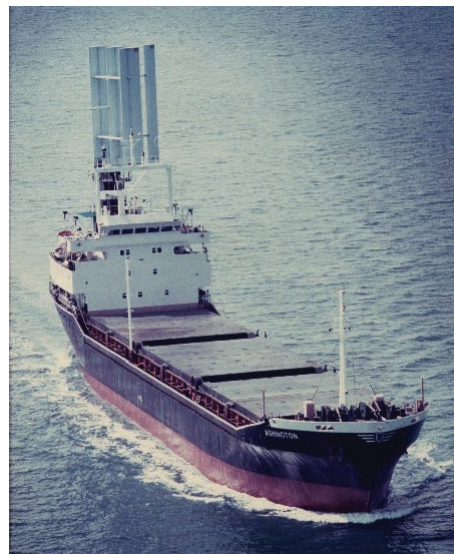
Figure 3.14 mv Ashington wing sail application © Mercator Media 2013
