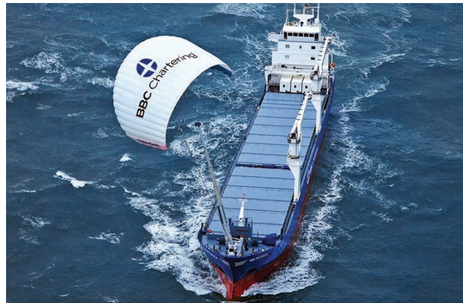
Figure 3.15 Application of a kite to assist propulsion © Sky Sails
